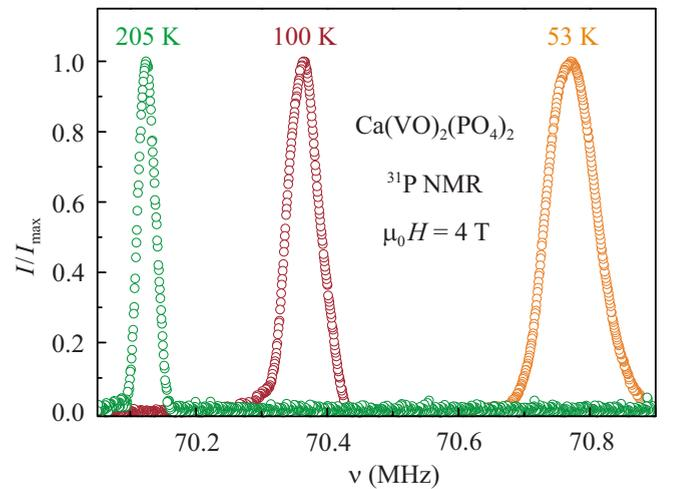
FIG. 7. (Color online)  $^{31}\text{P}$  NMR spectra for  $\text{Ca}(\text{VO})_2(\text{PO}_4)_2$  measured at 4 T by the Fourier transform of the spin-echo signal above  $T_N$ . The representative spectra show the line shift with temperature. All the spectra are normalized to unity by dividing the intensity ( $I$ ) by the maximum intensity ( $I_{\text{max}}$ ).
