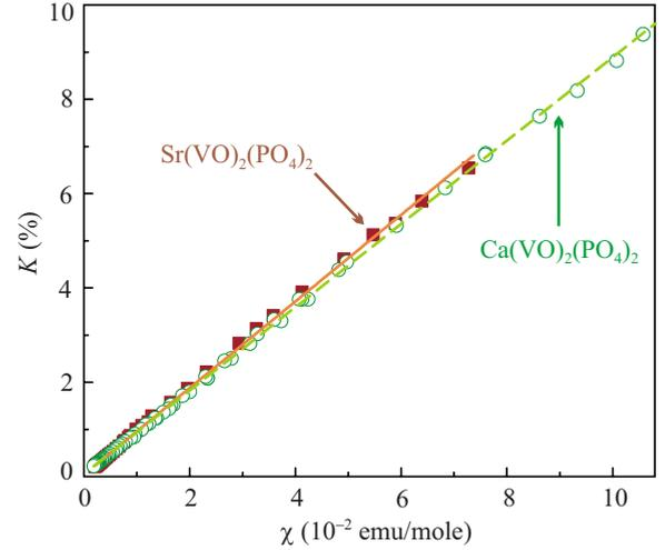
FIG. 9. (Color online)  $^{31}\text{P}$  NMR shift ( $K$ ) vs bulk susceptibility ( $\chi$ ) with temperature as an implicit parameter. We employ the  $\chi$  data collected at the applied field of 4 T since this field was used for the NMR measurements. The solid and dashed lines show the linear fits with Eq. (4).
