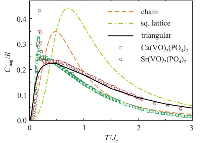
FIG. 5. (Color online) Magnetic contribution to the specific heat of  $M(\text{VO})_2(\text{PO}_4)_2$  and theoretical curves for the uniform chain (Refs. 30 and 34), nonfrustrated square lattice (Refs. 34 and 35), and triangular lattice (Ref. 34) models. The reduced temperature scale  $T/J_c$  with  $J_c = \sqrt{\sum_i J_i^2}$  is used.
