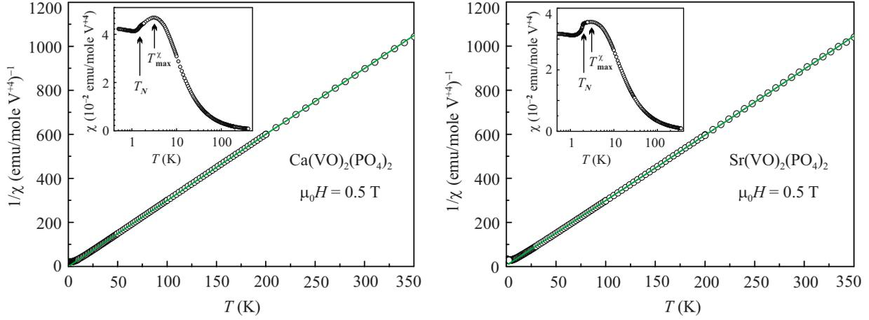
FIG. 2. (Color online) Reciprocal magnetic susceptibility ( $1/\chi$ ) vs temperature ( $T$ ) measured at  $\mu_0 H=0.5$  T down to 0.4 K for  $\text{Ca}(\text{VO})_2(\text{PO}_4)_2$  (left panel) and  $\text{Sr}(\text{VO})_2(\text{PO}_4)_2$  (right panel). The solid lines are best fits of the data to Eq. (1). In the insets,  $\chi$  vs  $T$  is plotted in the logarithmic scale to focus on the  $T_{\text{max}}^\chi$  and  $T_N$ .
