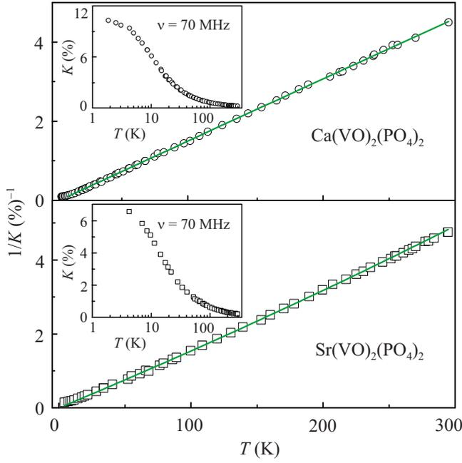
FIG. 8. (Color online) Inverse of  $^{31}\text{P}$  NMR shift ( $1/K$ ) vs  $T$  for  $\text{Ca}(\text{VO})_2(\text{PO}_4)_2$  (upper panel) and  $\text{Sr}(\text{VO})_2(\text{PO}_4)_2$  (bottom panel). Circles and squares indicate the experimental data, while the solid lines show the Curie-Weiss fits. The insets present the  $K$  vs  $T$  curves.
