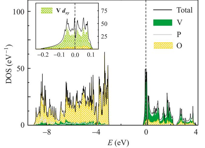
FIG. 11. (Color online) LDA density of states for Ca(VO)<sub>2</sub>(PO<sub>4</sub>)<sub>2</sub>. The Fermi level is at zero energy. The calcium contribution is negligible in the whole energy range; therefore it is not presented in the figure. The inset zooms the image near the Fermi level, only V  $3d_{xy}$  and oxygen contributions are shown.
