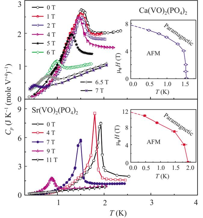
FIG. 6. (Color online) Specific heat of  $\text{Ca}(\text{VO})_2(\text{PO}_4)_2$  (upper panel) and  $\text{Sr}(\text{VO})_2(\text{PO}_4)_2$  (bottom panel) measured at different applied fields ( $H$ ). The insets show the respective  $H-T$  phase diagrams.
