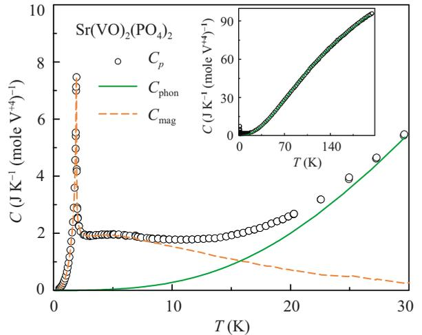
FIG. 4. (Color online) Temperature dependence of the specific heat measured at zero field for  $\text{Ca}(\text{VO})_2(\text{PO}_4)_2$  (left panel) and  $\text{Sr}(\text{VO})_2(\text{PO}_4)_2$  (right panel). The open circles are the raw data, the solid lines show the phonon contribution  $C_{\text{phon}}$  as found from the fit to Eq. (2), and the dashed lines denote the magnetic contribution  $C_{\text{mag}}$ . The insets show the fits with Eq. (2) in the wide temperature range.
